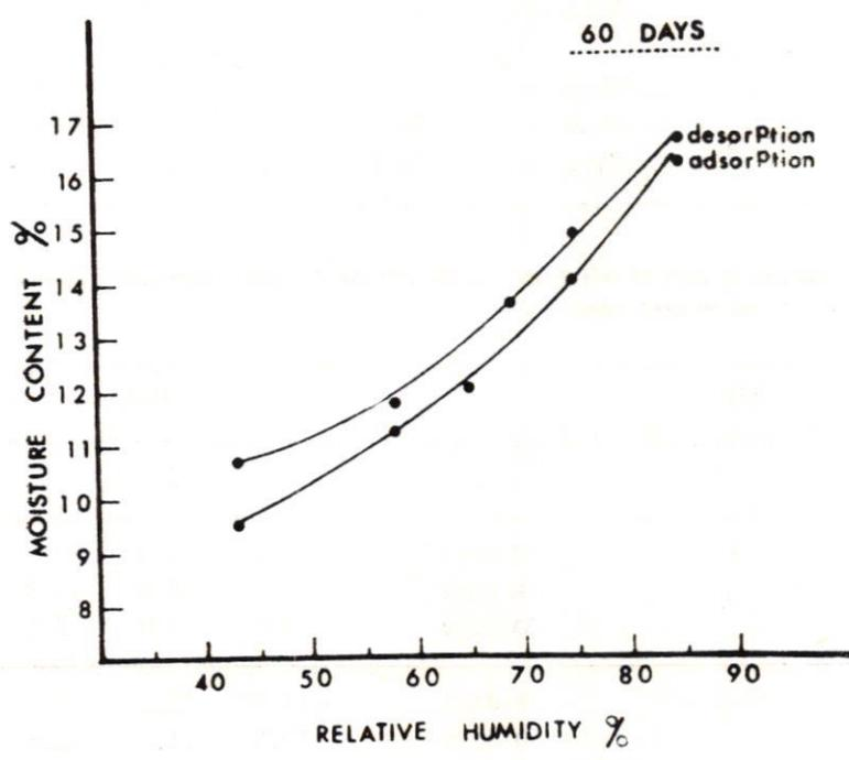
Fig. 1 Moisture content/relative humidity equilibrium of hard wheat at 27°C, showing desorption and adsorption curves
