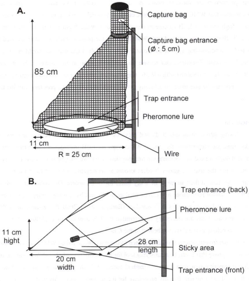
**Fig. 1-** Traps design used for male European Corn Borer capture.
